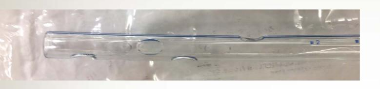
Tip, with drainage holes and "sentinel eye".
