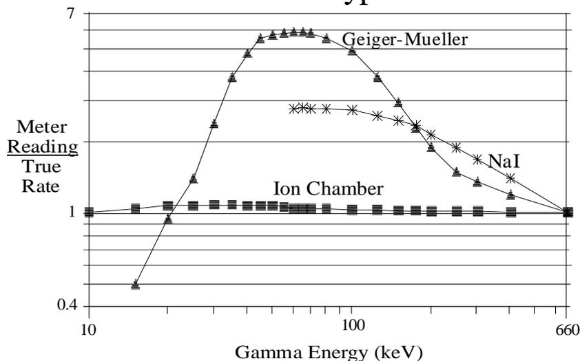
*Energy Dependence:* Radiation detection instruments are not equally accurate at measuring all radiation energies, as shown by the graph. All instruments were calibrated to be accurate at 660 keV.
