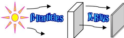
Figure 1. Shielding arrangement for large quantities of high energy  $\beta$ -emitting radionuclides to eliminate exposure due to Bremsstrahlung radiation by first using a low-Z material immediately followed by a high-Z material.
