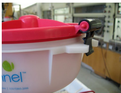
Example of Improper Closure of funnel
