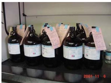
Improper Hazardous Waste Storage. No secondary containment from hood drain, storage in high traffic area.
