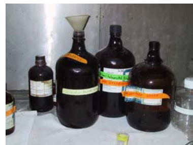
Improper Hazardous Waste Storage. No OCRS labels, no secondary containment, and container not sealed properly (open funnel).
