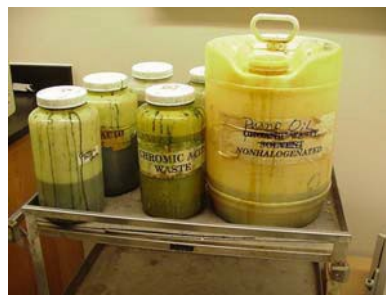
Improper Hazardous Waste Storage. No OCRS labels, no secondary containment, no segregation, and containers are covered with residue.
