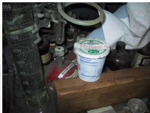
Example of Improper use of a Food Grade Container for hazardous material storage
