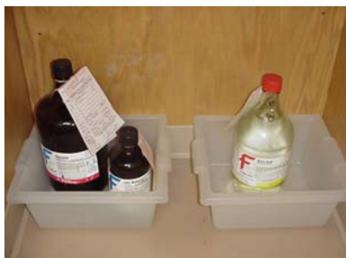
Proper Hazardous Waste Storage. Hazardous waste is labeled, segregated by compatibility, stored in secondary containment, and in an isolated area.
