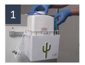
Place new cartridge in cage with FRONT facing outward. Put cap in cage on right side of cartridge.
