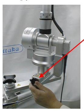
Set up Point Setter arm. Make sure that the arm is securely clamped to the OR table adapter.
