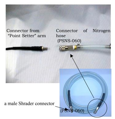
Plug the arm hose into the nitrogen connector of the hospital. Set pressure to  $6 \sim 8$  kg/cm or 90  $\sim 115$  psi.
