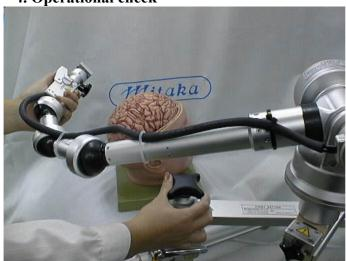
Perform operational check of the Point Setter and make sure the range of motion is appropriate. Do this before starting surgery.
