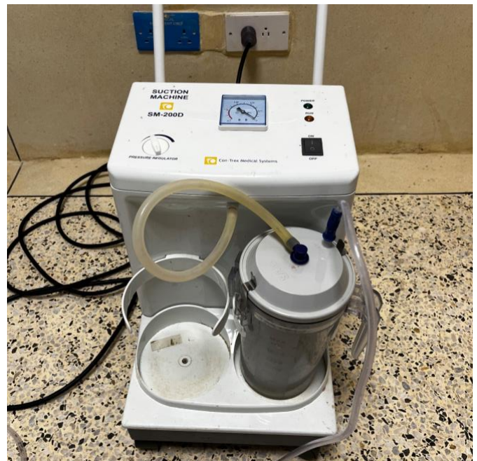
A wall-powered portable suction machine. Note that this machine runs on 110 volts and needs a separate outlet, as it is being used in a country where 220 volts (Blue outlet) is more commonly used.
