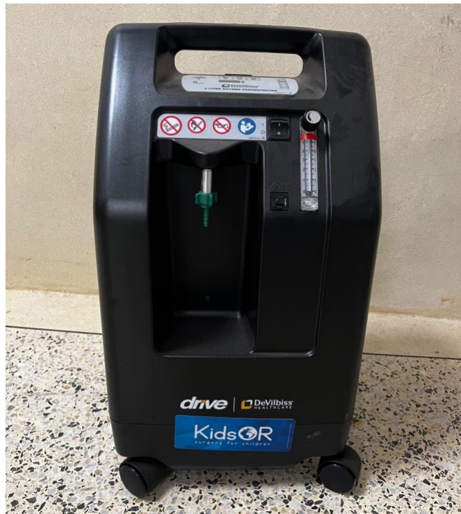
A portable, wall-powered oxygen concentrator
