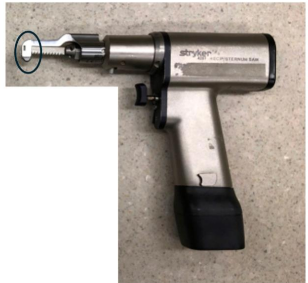
Electrical saw with sternotomy attachment. The “guard” in the Black circle is meant to sit under the sternum while the blade cuts the bone: the surgeon pulls the guard up against the bone by pulling upward on the handle, to prevent the blade from cutting anything deeper.
