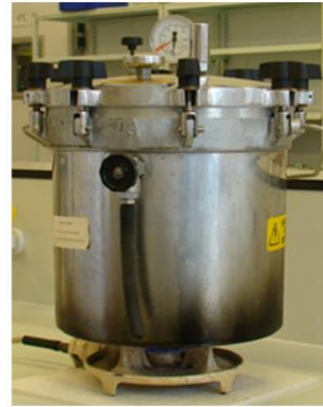
A simple electric pressure cooker autoclave. Source: Viv Rolfe, CC BY-SA 4.0
