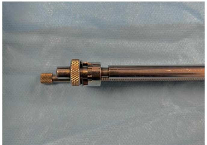
Adjustments to the thickness of the blade are made by turning the dial. On some models of the Humby knife, there is another dial that secures the thickness once the adjustment has been made.
