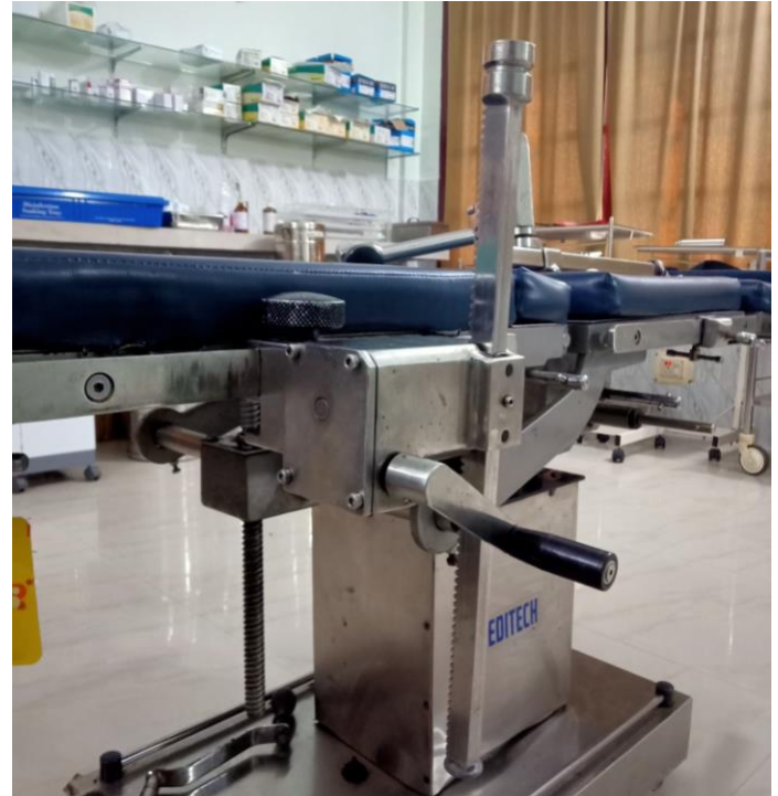
Part that attaches to the Operating Table. There is a "V" shaped cut that allows the clamp to attach to any operating table, and the screws fix it tight. The vertical portion should start low so that once the lift is set up, it can be rotated.
