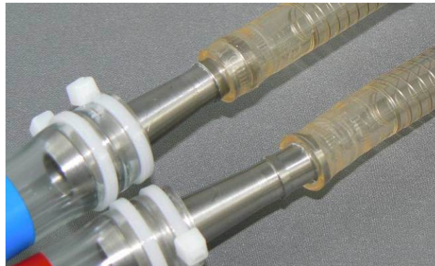
Figure 16-2 – Metal Hose Barb Connectors Loosened, but Still Connected, to the Cannulae
